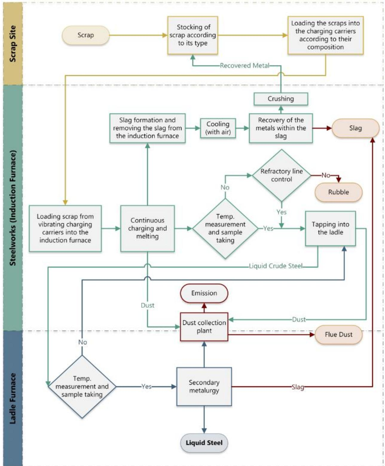
Figure 1 Bilecik Iron and Steel Works Industry and Trade Co. (BDÇ) Production Flow Chart for LS
